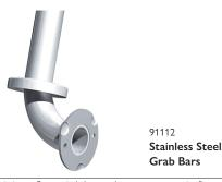
Description: Features include cover that snaps over mounting flange dimples to conceal screws and concealed mounting flange of 3-1/8 (79 mm) O.D. diameter with 2 screw holes and 3 locking dimples; 1/8 (3 mm) thick, type 304 stainless steel. Cover is type 304 stainless steel with a satin finish and 22 gauge; 3-3/16 (81 mm) diameter.
